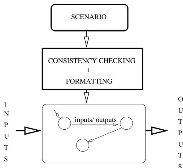
**Figure 3. The state machine for the constraint-based approach**
