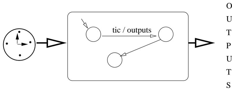
**Figure 4. Input of the state machine associated with a absolute temporal axis**
